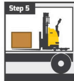
Stacker's legs slide to the front.
