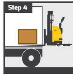
Stacker lifts itself using a reverse lift motor.
