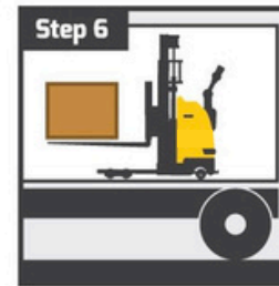
Stacker truck & load safely in the truck for unloading later using the same method.
